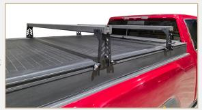
Insert a T Nut into the Rack Crossbar T-Slot, thread in a Wing Bolt, and tighten as pictured. Do this on all (4) 6" Side Arms.
